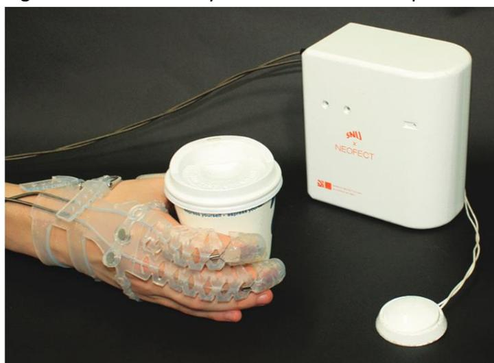
Kang, B. B., Choi, H., Lee, H., & Cho, K.-J. (2019). Exo-Glove Poly II: A Polymer-Based Soft Wearable Robot for the Hand with a Tendon-Driven Actuation System. *Soft Robotics*, 6(2), 214–227. <https://doi.org/10.1089/soro.2018.0006>
