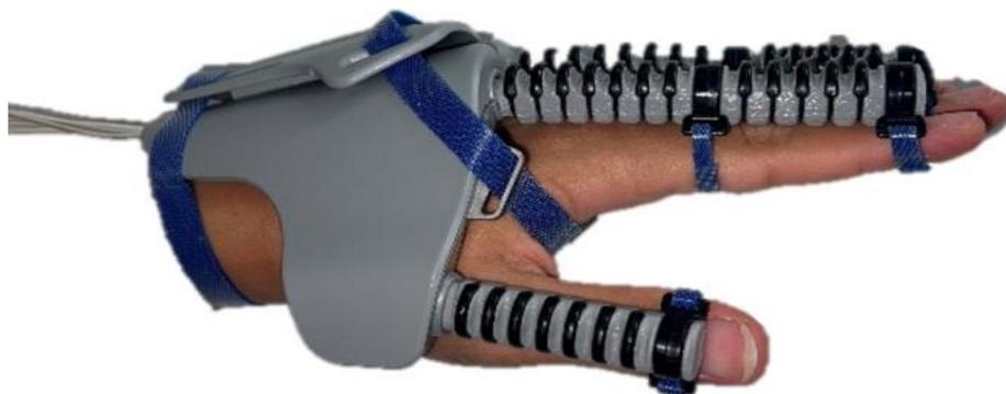
Zhou, C.-Q., Shi, X., Li, Z., & Tong, R. K.-Y. (2022). 3D Printed Soft Robotic Hand Combining Post-Stroke Rehabilitation and Stiffness Evaluation (pp. 13–23). [https://doi.org/10.1007/978-3-031-13835-5\\_2](https://doi.org/10.1007/978-3-031-13835-5_2)
